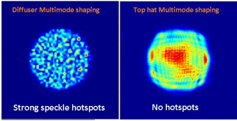
illumination is required over a certain depth of of focus, such as in the case of frequancy conversion crystals. Diffuser type solutions, such as Micro lens arrays and <u>diffractive diffusers</u>, are often used in such cases ,but tend to generate speckle if the laser is somewhat coherent and thus create hotspots on the optical components, shortening system lifetime and requiring costly maintainance visits.
