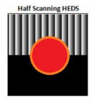
The growth of Laser welding is leading to many challenging applications, including cases of butt-joint welding where only the two sides of the weld must be heated, with no power dposited in the middle. While our standard 1X2 DS beam splitters have typical zero order energies of <0.5% of input, this is still too much for such applications.
