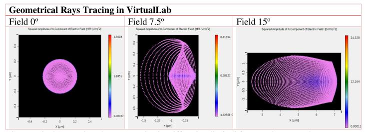
Geometrical raytracing shows spot size is Diffraction limited for tested scan angles.
