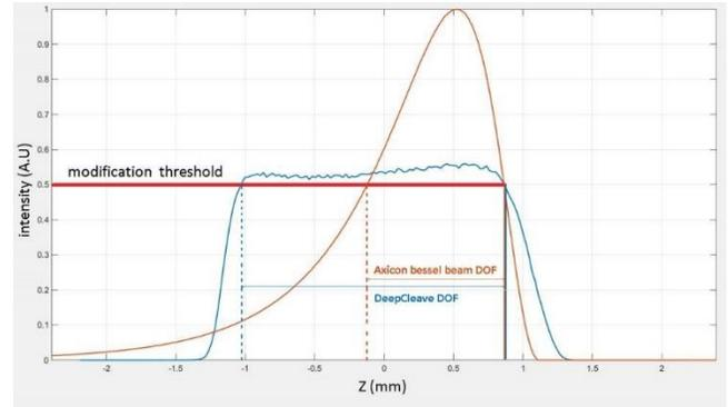
The required hole diameters are decreasing with advances in miniaturization , requiring a method of focusing the laser very tight spots with depth of focus equal to the glass thickness. Here, our DeepCleave modules shine!
