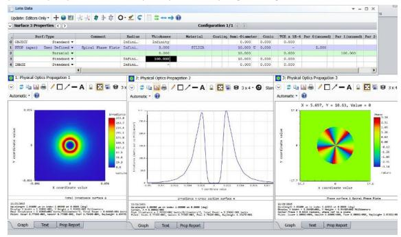
Notes: The effect of the Vortex Phase Plate can be seen only with Physical Optics Propagation
