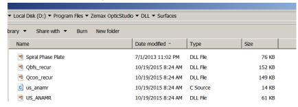
2. The DLL file should be loaded in "User Defined" surface and the user must enter the OAM charge (Topological charge) value into the first parameter of the surface.
