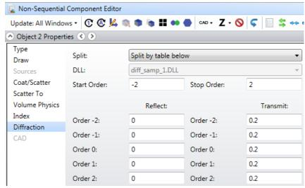
For even number of foci activated orders will be: -n+1 to n-1 with step 2. For example multifocal lens with 4 foci n = 4, "Start Order" is -3, and "Stop Order" is 3.
