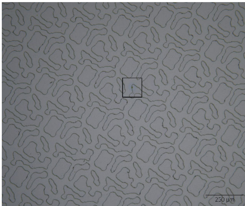
Figure 5. Typical damage morphology: fluence 28.2 J/cm 2 , damage after 1000 pulse(s).
