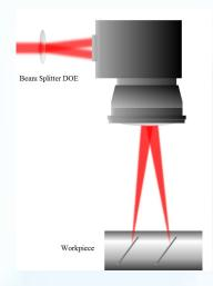
This way, the beam can be splited to as many spots as desired, with accurately defined separations, without the need for extra costly and bulky write heads, with separate scanners.
