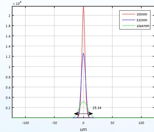
As can be seen above, peak power for the diffractive Achromat is ~ X3 higher than the YAG-BBAR refractive Achromat corrected for 500-1100nm and is ~ X25 higher than the UV-to-NIR Corrected Triplet.
