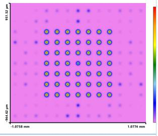
Intensity result of Beam Splitter 7x7 binary type
