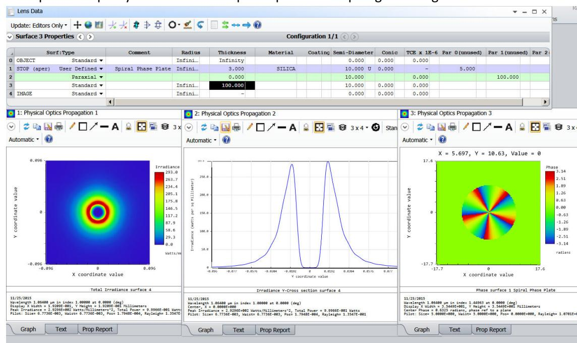
**Notes:** The effect of the Vortex Phase Plate can be seen only with Physical Optics Propagation
